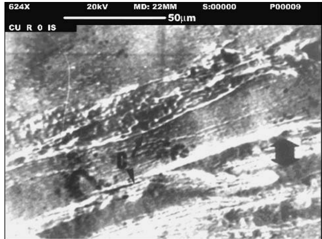
Fig. 7 Scanning electron micrograph of a flow band seen at 298 K and 1 \text{ s}^{-1} . Cracks at flow band boundaries (marked by arrows and “c”) can be seen.
